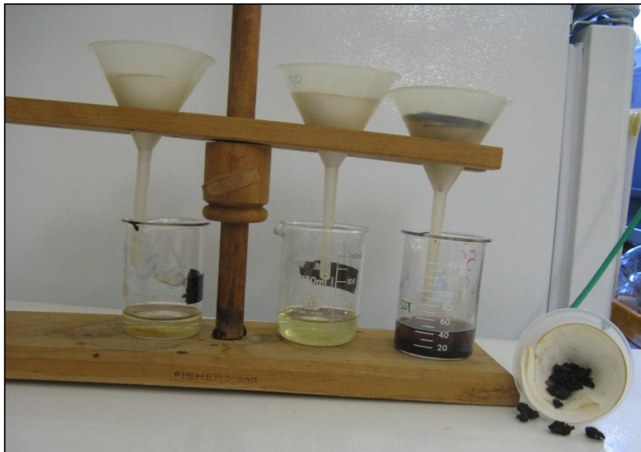
Figure 12. The funnels set up, with increasing pH of extractant from left to right.
