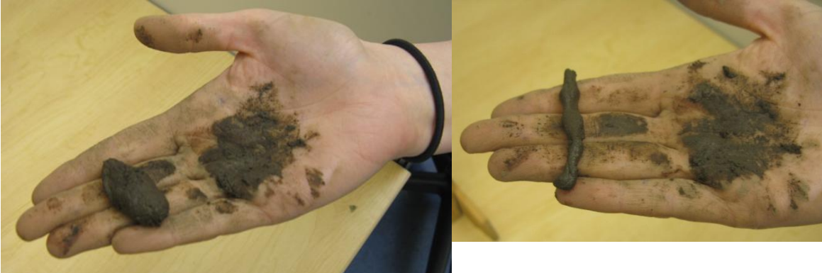
Figure 1. The student above has made a ball/cast of the soil (left) and a worm (right) to test for differences in soil texture.
